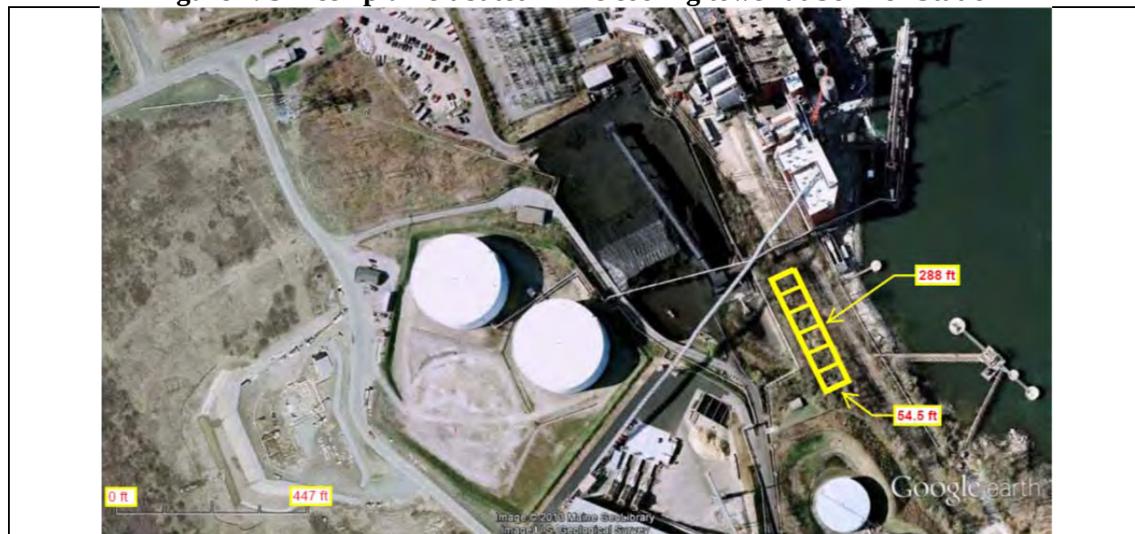
Figure 2. Six-cell plume-abated inline cooling tower at Schiller Station
